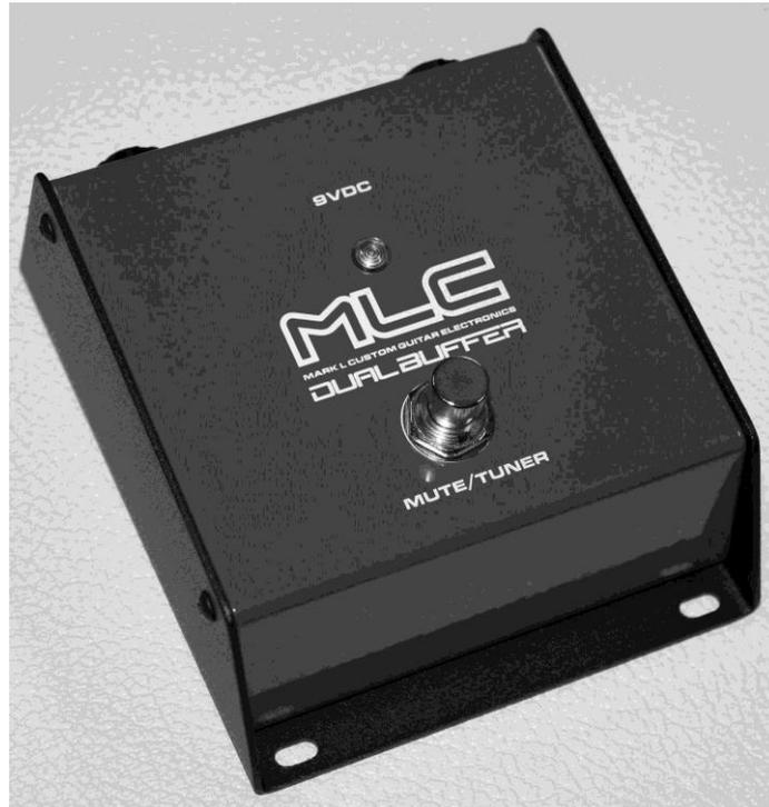
**MLC DUAL BUFFER** has been specifically designed to overcome the problems often encountered with amplification of Electric Instruments fitted with magnetic transducers. The usual cause of these problems is the mismatch of the impedance in the electrical circuit between the pickup and subsequent equipment.
